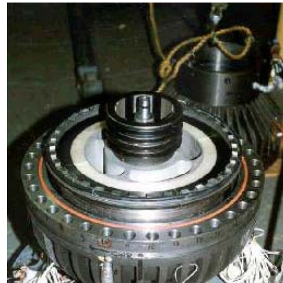
TSI FESS with safety cap removed
